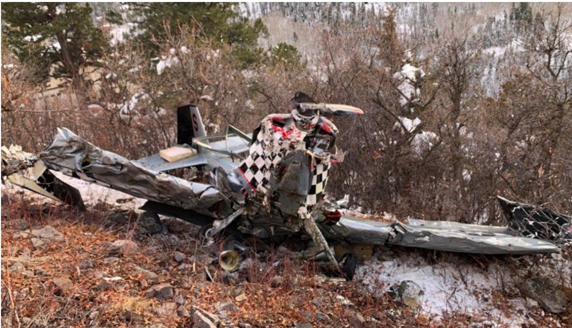
Figure 1. Wreckage of an RV-4 destroyed after a low-speed loss of control during base to final turn. The ATP-rated pilot and non-pilot passenger were killed [4]. Experimental aircraft are not required to have stall warning.
